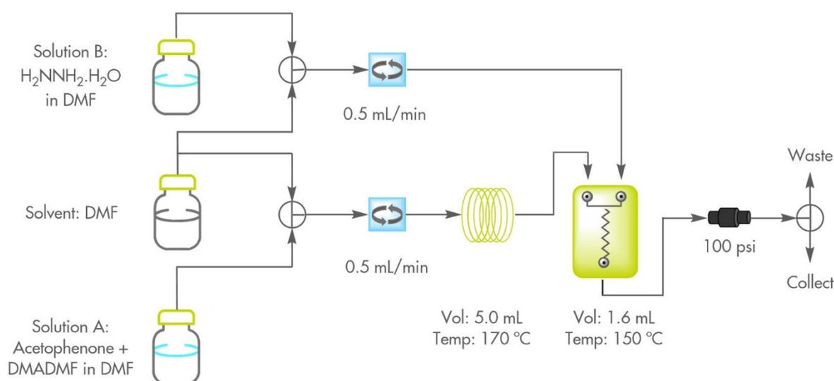
**Scheme 2** Schematic of the flow system set-up.
